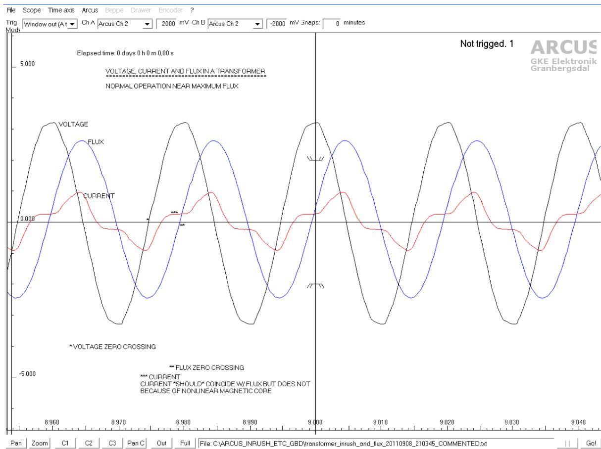
Normal operation. Note distorted current (red) while flux (blue) is sine shaped.
