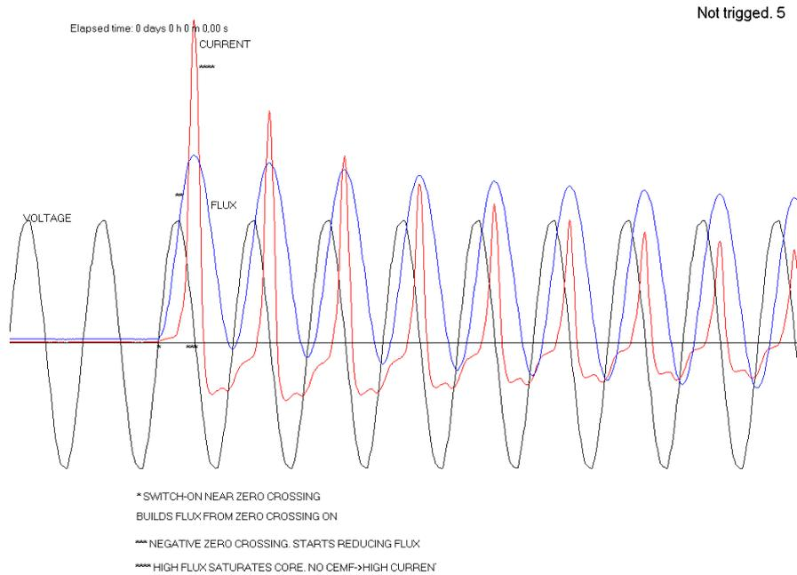
In this picture, voltage switch-on is near the zero crossing. That means that flux starts from zero instead of maximum negative flux, which means that it reaches saturation earlier and therefore causes an increased inrush current.
