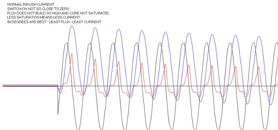
Some distance from zero reduces inrush current. Best is 90 degrees, but that needs special relays (SSR) with the corresponding synchronization and delay. They are available but not commodities like zero-crossing relays.
